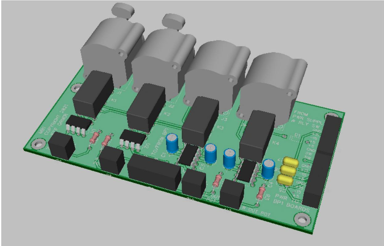
The MB1 is used in the TPC-100 Prism clone to translate balanced +4dBu studio level audio to unbalanced audio with the ability to bypass the balanced inputs when powered off or by use of a switch. There are provisions for input and output level pots as well as power distribution to the BP1 processor boards. A connection allows switching for relay bypass.
